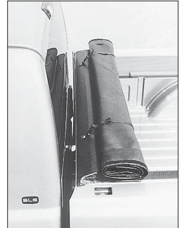
Cover rolled fully open with both safety straps secured. NOTE: Cover is not rolled against cab to avoid wear on paint and cover.
