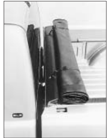
Cover rolled fully open with both safety straps secured. NOTE: Cover is not rolled against cab to avoid wear on paint and cover.
