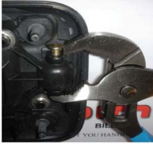
16) Remove the front pin with pressure as shown above
