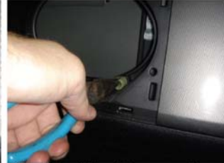
6) pull straight out to remove lower nylon speaker nut inserts
