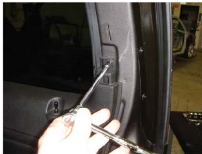
5a) remove 6 mm bolt at the top rear of the door panel and go to step 7 above
