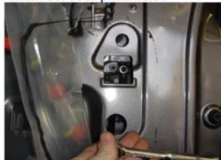
13) Remove 2 10 mm nuts on the front inside of the door handle
