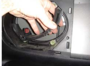
5) remove lower speaker seal
