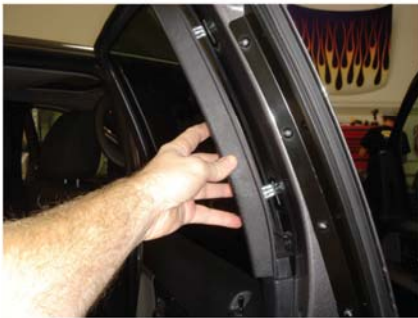
4a) on the rear door, unclip the trim panel
