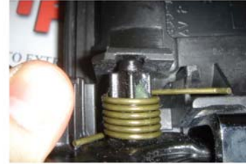
18) remove latch and handle
