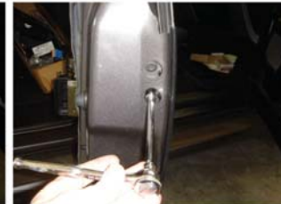
12) remove 2ea 10 mm bolts at rear of door handle
