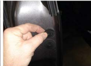
11) remove 2 plugs at rear of door
