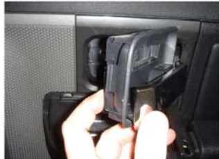
10) Lift off door panel & unclip latch. Set door panel aside
