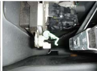
14) release the latch rod at the base with the quick (dis)connector
