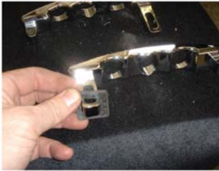
19) remove the rubber pad from the original handle and install on the Grippin Billet Handle
