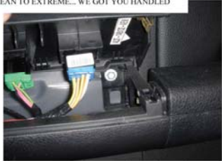
1) Pry up switch panel and unclip
