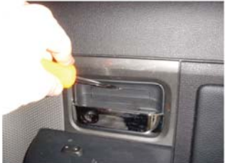
7) Remove inside latch cover panel
