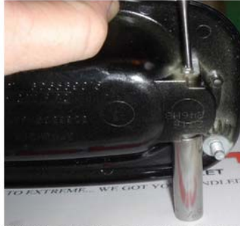
20) drive the pin out using a socket to receive the pin
