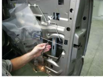
17) remove the front 10mm bucket nut
