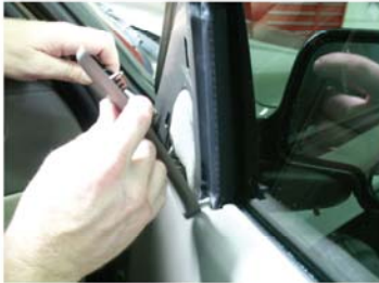
2) unclip top front panel
