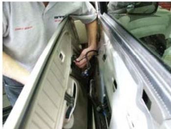
11) unplug any remaining wires
