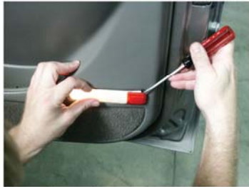
5) unclip and unplug courtesy light
