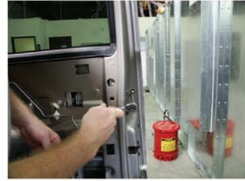
15) carefully remove 10 mm nut
