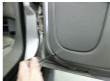
10) remove lower door panel bolt
