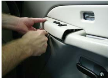
7) 1999-2001 ONLY-unclip switch panel
