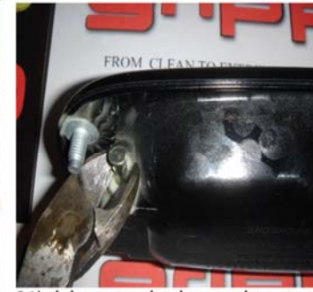
21) dykes can also be used to extract the front pivot pin
