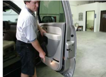
12) lift the door panel up and off
