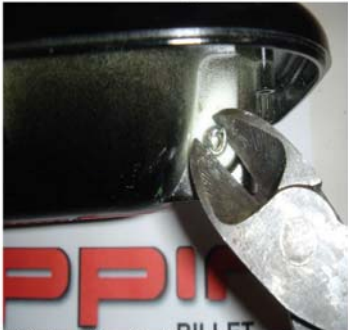
19) nip off soft alloy pin head
