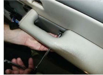
6) remove 7 mm bolt behind pull handle
