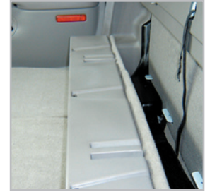
The DU-HA bolts to rear floor flaps to allow access to the jack when tilted forward.
